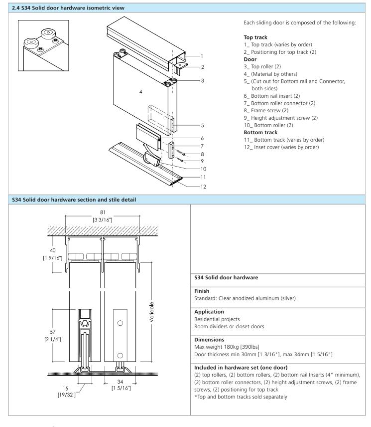
System description\_ S34\_ S150, S300, S720, Solid Door Hardware Sliding door system
